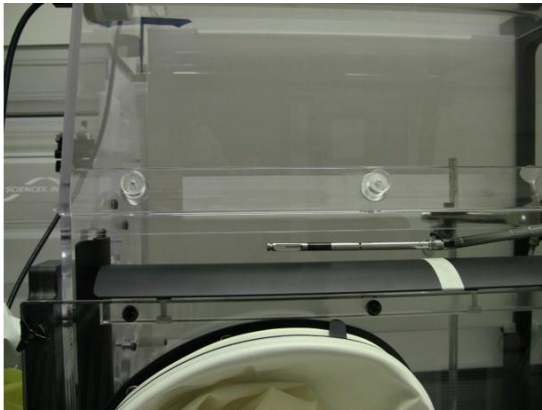
Place anemometer tip in the plane of the face opening. Measure values above and below draft shield.
