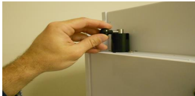
Pull filter clamps up and rotate to release primary HEPA filter
