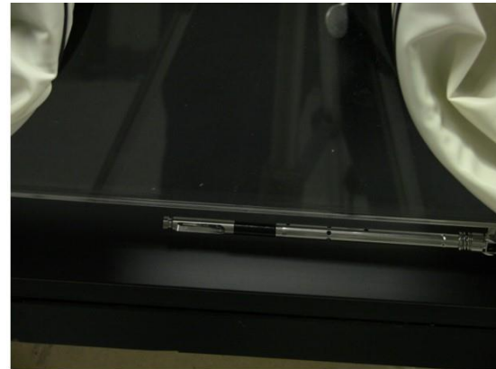
Place anemometer tip in the plane of the face opening. Measure values above and below draft shield.
