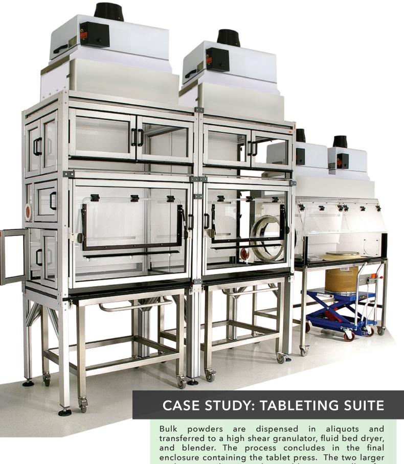
Bulk powders are dispensed in aliquots and transferred to a high shear granulator, fluid bed dryer, and blender. The process concludes in the final enclosure containing the tablet press. The two larger enclosures utilize interchangeable carts to allow for other pieces of equipment to be accommodated as desired. Units include dual Bag In/Bag Out HEPA filtration for maximum containment. Surrogate sampling showed containment results of 1 to 5 mg/m3.
