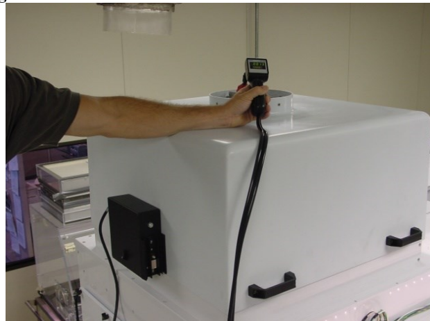
Fig. 50. Measure at Exhaust Port
