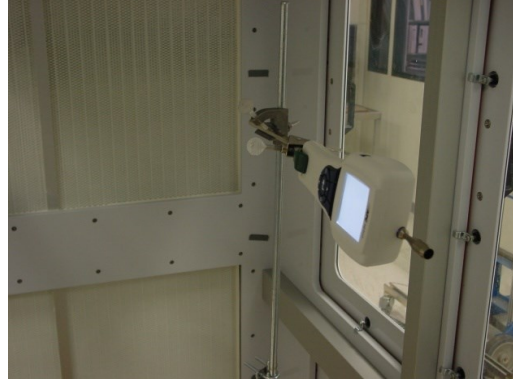
Fig. 52. Particle Counter Facing Airflow
