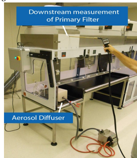
Fig. 37. Downstream Measurement Location
