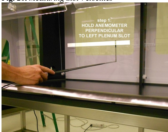
Fig. 20. Measuring Slot Velocities
